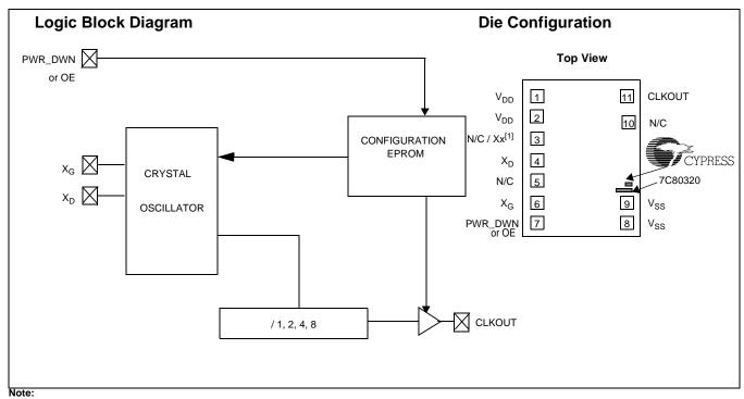
1. For customers not bonding  $X_D$  or  $X_G$  pad to external pins, an alternative bonding option would be shorting the Xx pad to the  $X_D$  pad.
