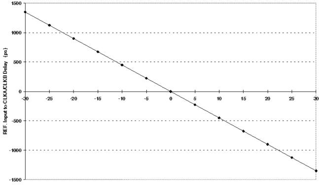
Output Load Difference: FBK Load - CLKA/CLKB Load (pF)
