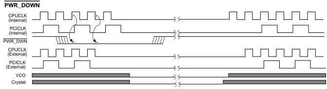
Shaded section on the VCO and Crystal waveforms indicates that the VCO and crystal oscillator are active, and there is a valid clock.
