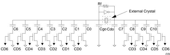
CD = EPROM BIT T = TRANSISTOR C = LOAD CAPACITOR
