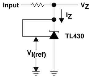
Figure 1. Test Circuit for  $V_Z = V_{I(ref)}$
