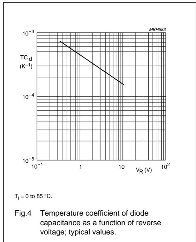
Low-voltage variable capacitance diode
