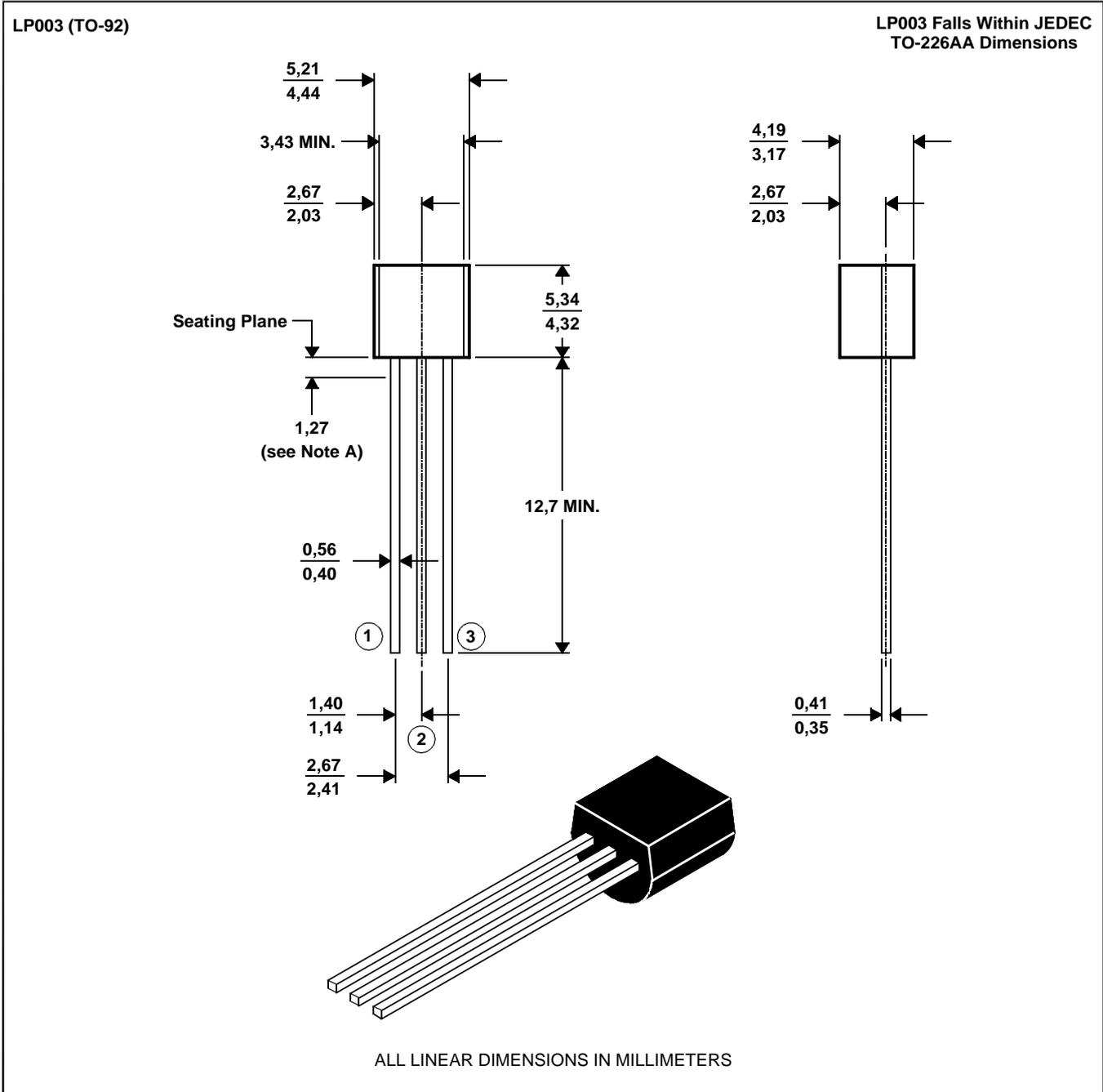
NOTE A: Lead dimensions are not controlled in this area.
