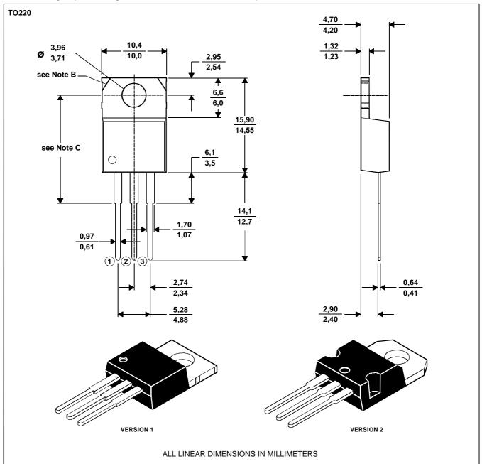
NOTES: A. The centre pin is in electrical contact with the mounting tab.
