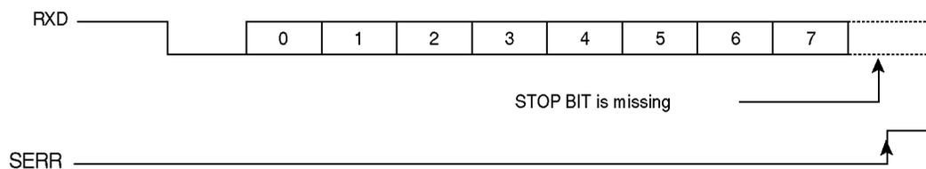
In this example the receiver waits for a STOP BIT to complete the frame reception. Unfortunately the stop bit isn't there and the receiver indicates the frame error by setting to 1 the SERR bit in the IOCON register.
