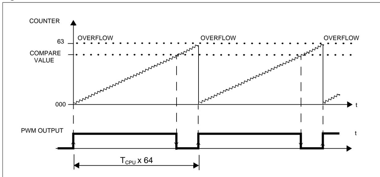
The counter increments continuously, clocked at internal CPU clock. Whenever the 6 least significant bits of the counter (defined as the PWM counter) overflow, the output level for all active channels is set.
