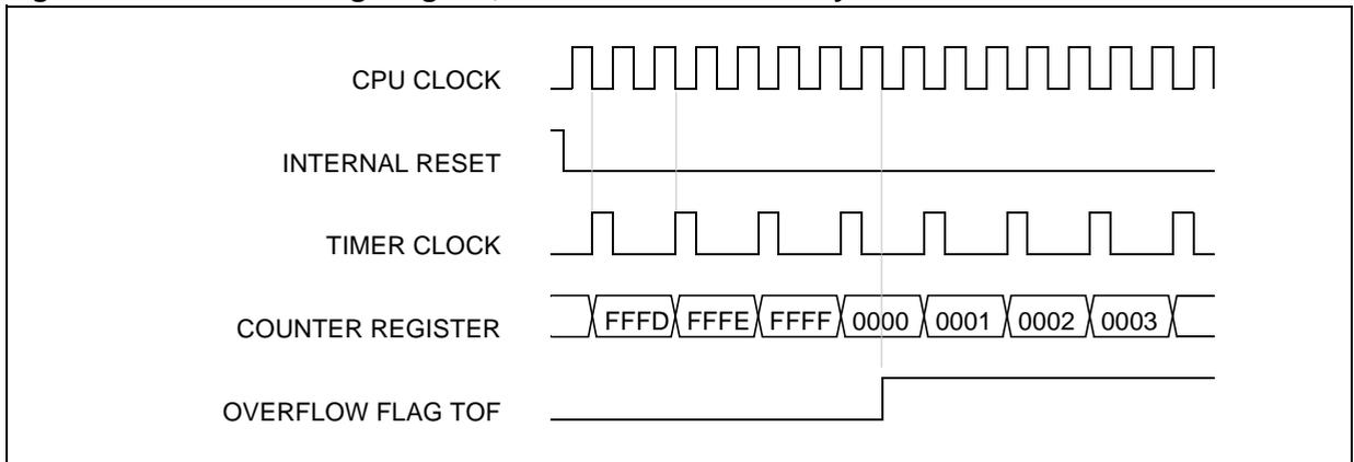
Figure 19. Counter Timing Diagram, internal clock divided by 4
