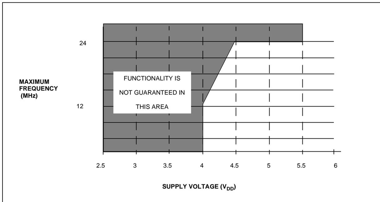
**Note:** The shaded area is outside the recommended operating range; device functionality is not guaranteed under these conditions.
