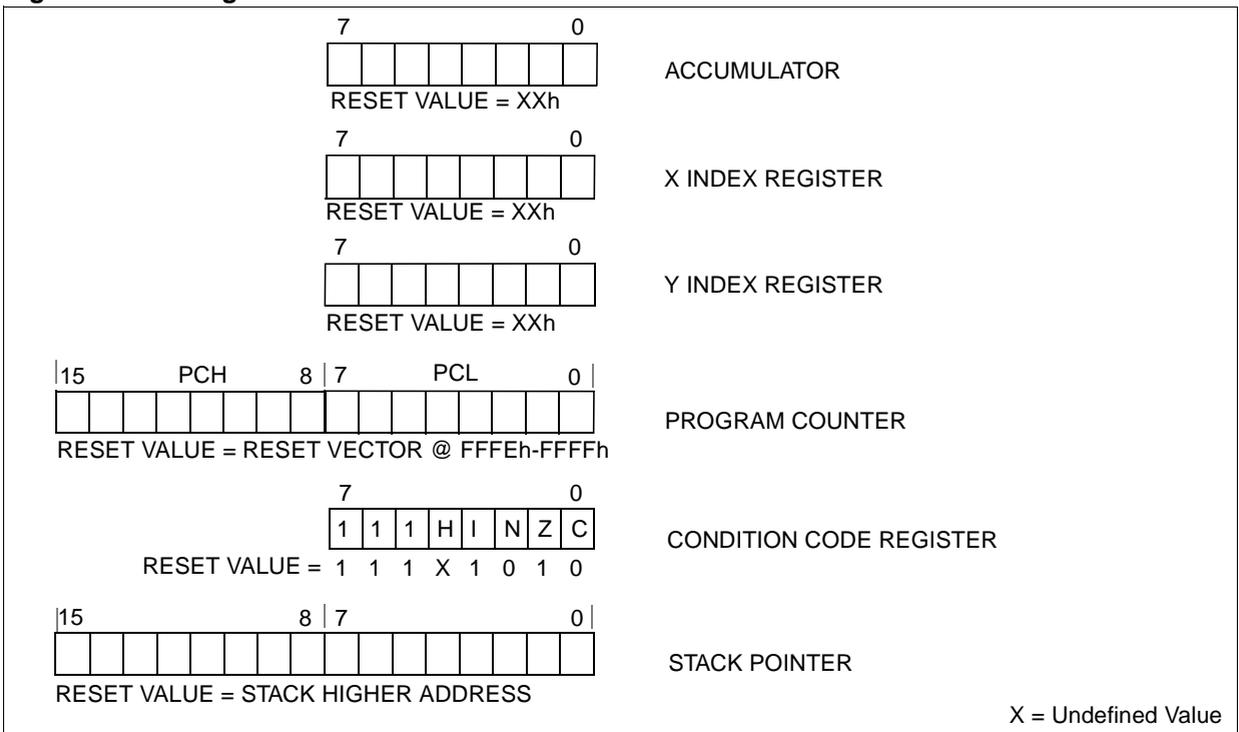
**CENTRAL PROCESSING UNIT (Cont'd)****Condition Code Register (CC)**
