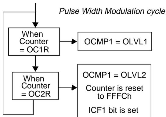
**Note:** After a write instruction to the OC/R register, the output compare function is inhibited until the OCLR register is also written.
