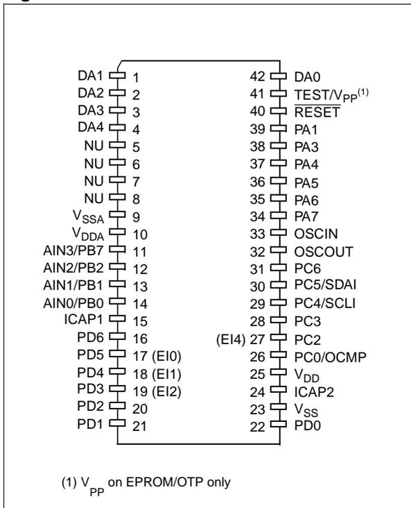
**Note:** Several pins of the I/O ports assume software programmable alternate functions as shown in the pin description.
