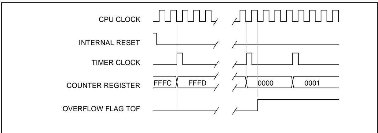
Figure 20. Counter Timing Diagram, internal clock divided by 8
