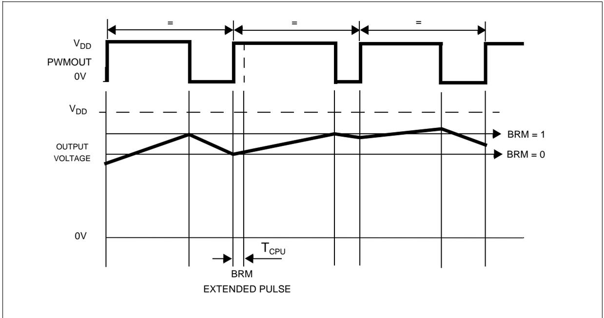
Figure 36. Graphical Representation of 4-Bit BRM Added Pulse Positions
