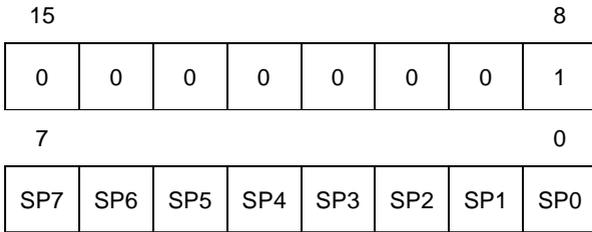
The Stack Pointer is a 16-bit register which is always pointing to the next free location in the stack. It is then decremented after data has been pushed onto the stack and incremented before data is popped from the stack (see Figure 7).
