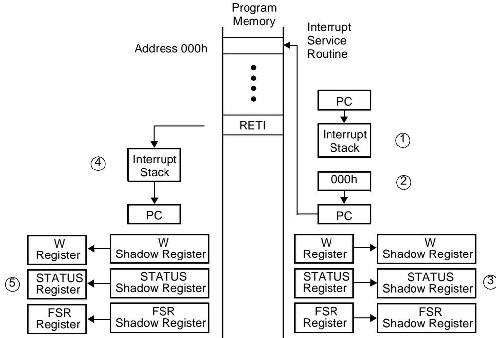
Note: The interrupt logic has its own single-level stack and is not part of the CALL subroutine stack.
