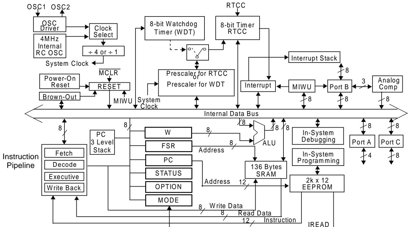
Figure 1-1. Block Diagram
