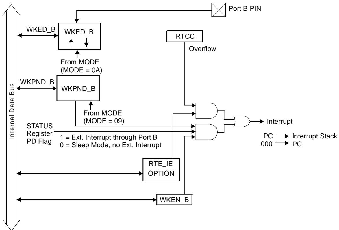
Figure 8-1. Interrupt Structure
