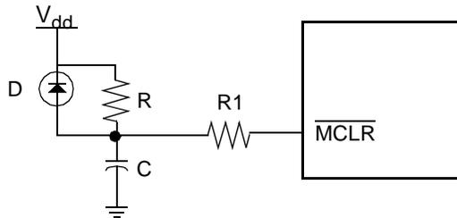
**Figure 12-5. External Power-On Reset Circuit (For Slow V<sub>dd</sub> Power-up)**
