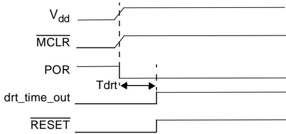
**Figure 12-3. Time-out Sequence on Power-up (MCLR tied to V<sub>dd</sub>): Fast V<sub>dd</sub> Rise Time**
