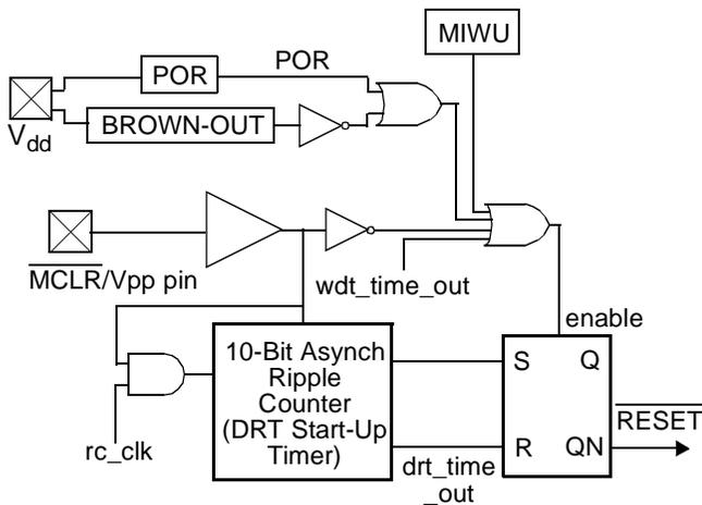
Note: Ripple counter is 10 bits for Power on Reset (POR) only.
