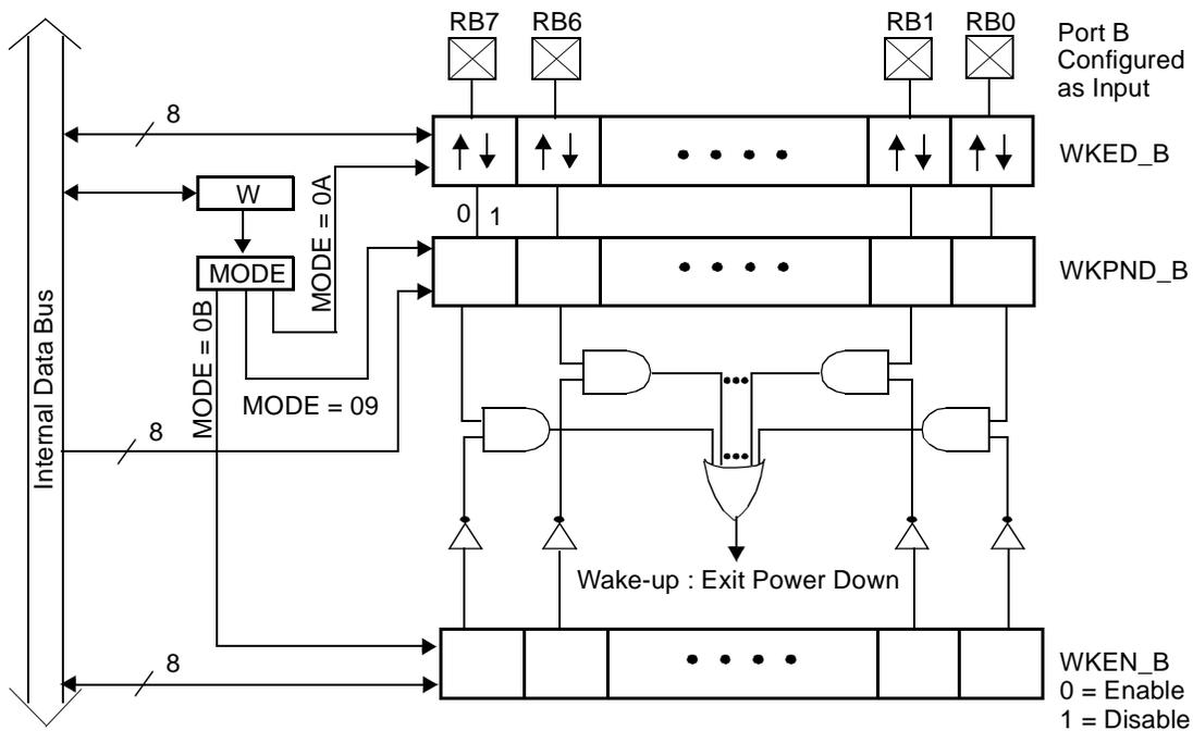
Figure 7-1. Multi-Input Wakeup Block Diagram
