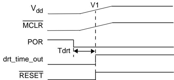
**Figure 12-4. Time-out Sequence on Power-up (MCLR tied to V<sub>dd</sub>): Slow Rise Time**
