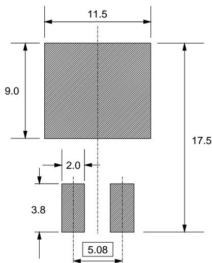
Fig.8. SOT404 : minimum pad sizes for surface mounting.
