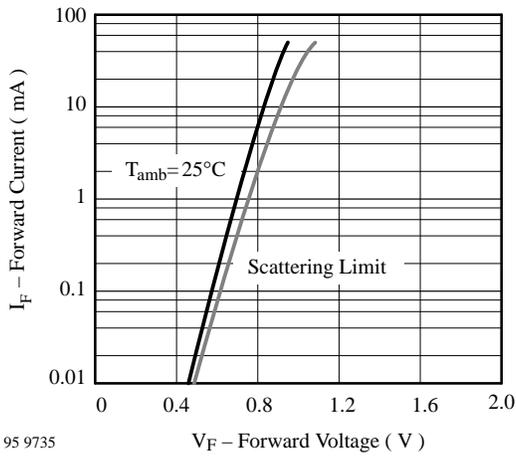
Figure 1 : Forward Current vs. Forward Voltage
