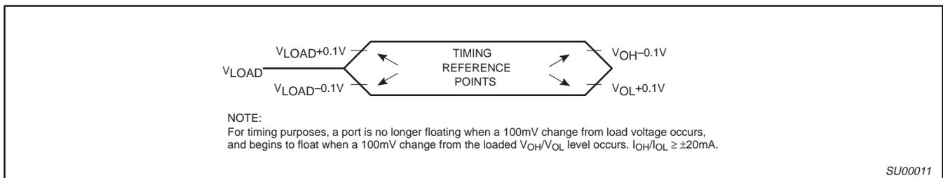
Figure 8. Float Waveform
