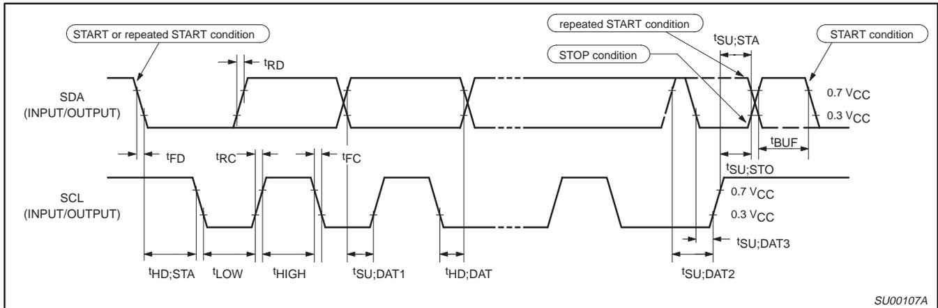
Figure 6. Timing SIO1 (I<sup>2</sup>C) Interface
