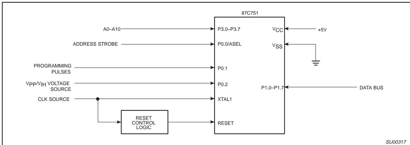
**Figure 5. Programming Configuration**
