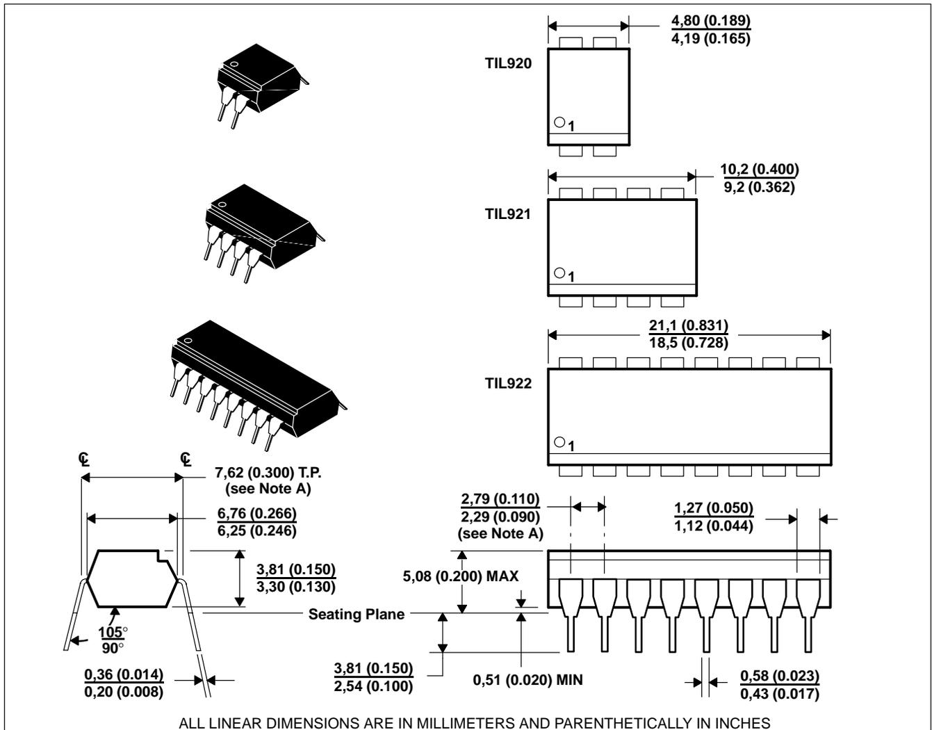
NOTE A: Each pin centerline is located 0,25 (0.010) of its true longitudinal position.
