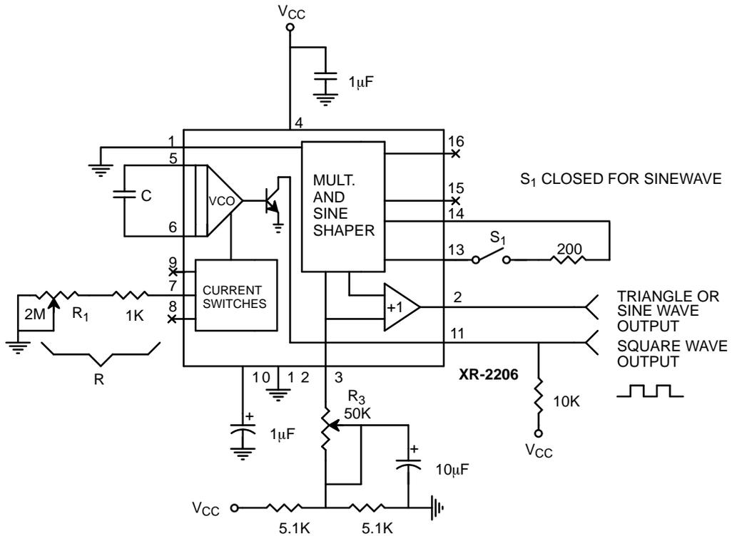
**Figure 11. Circuit for Sine Wave Generation without External Adjustment.**
