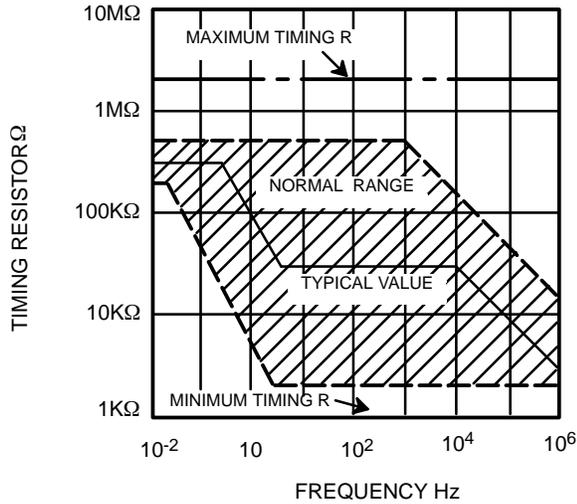
**Figure 5. R versus Oscillation Frequency.**
