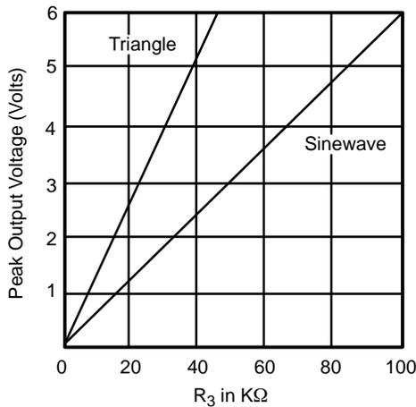
**Figure 3. Output Amplitude as a Function of the Resistor, R<sub>3</sub>, at Pin 3.**
