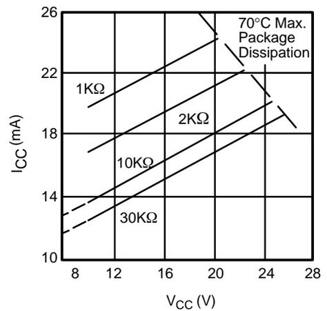
**Figure 4. Supply Current vs Supply Voltage, Timing, R.**
