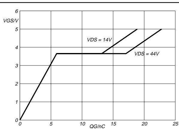
Fig.13. Typical turn-on gate-charge characteristics.
