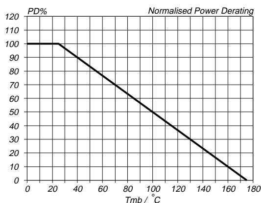
Fig.1. Normalised power dissipation.
