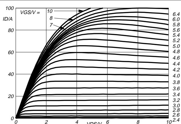
Fig.5. Typical output characteristics,  $T_j = 25^\circ\text{C}$ .
