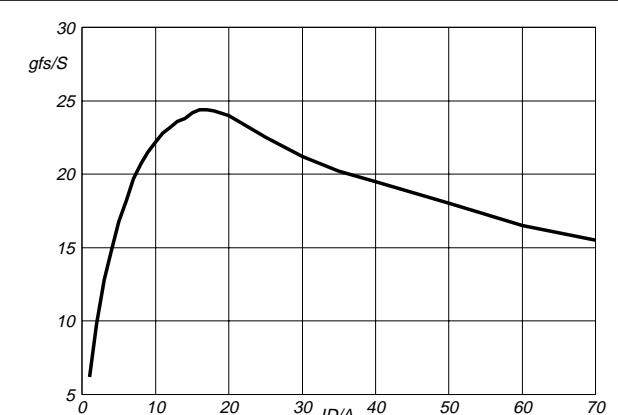
Fig.8. Typical transconductance,  $T_j = 25^\circ\text{C}$ .
