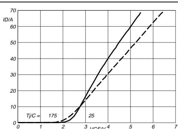
Fig.7. Typical transfer characteristics.
