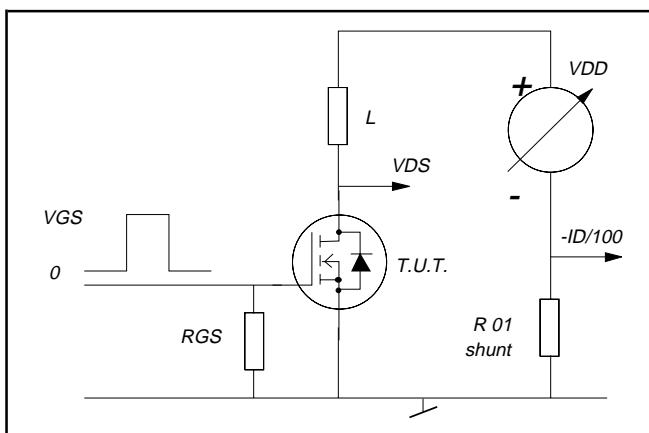
Fig.16. Avalanche energy test circuit.
