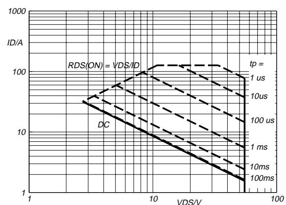
Fig.3. Safe operating area.  $T_{mb} = 25^\circ\text{C}$
