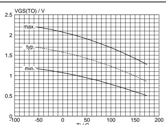
Fig.10. Gate threshold voltage.
