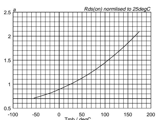
Fig.9. Normalised drain-source on-state resistance.
