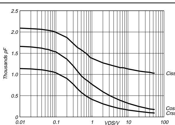
Fig.12. Typical capacitances,  $C_{iss}$ ,  $C_{oss}$ ,  $C_{rss}$ .
