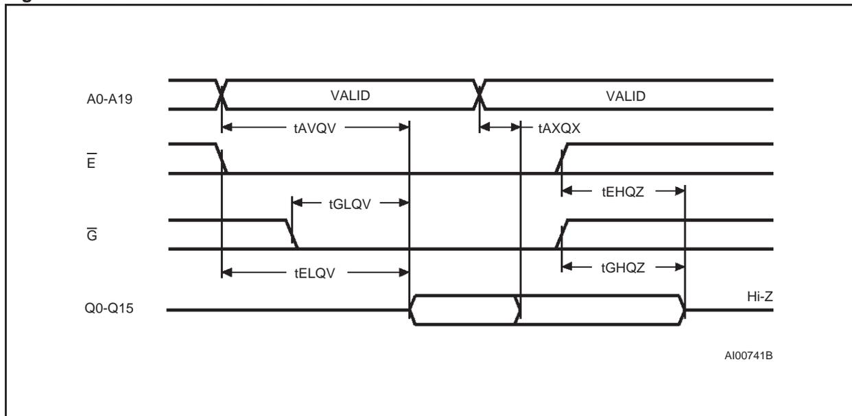
Note:  $\text{BYTE } V_{PP} = V_{IH}$ .
