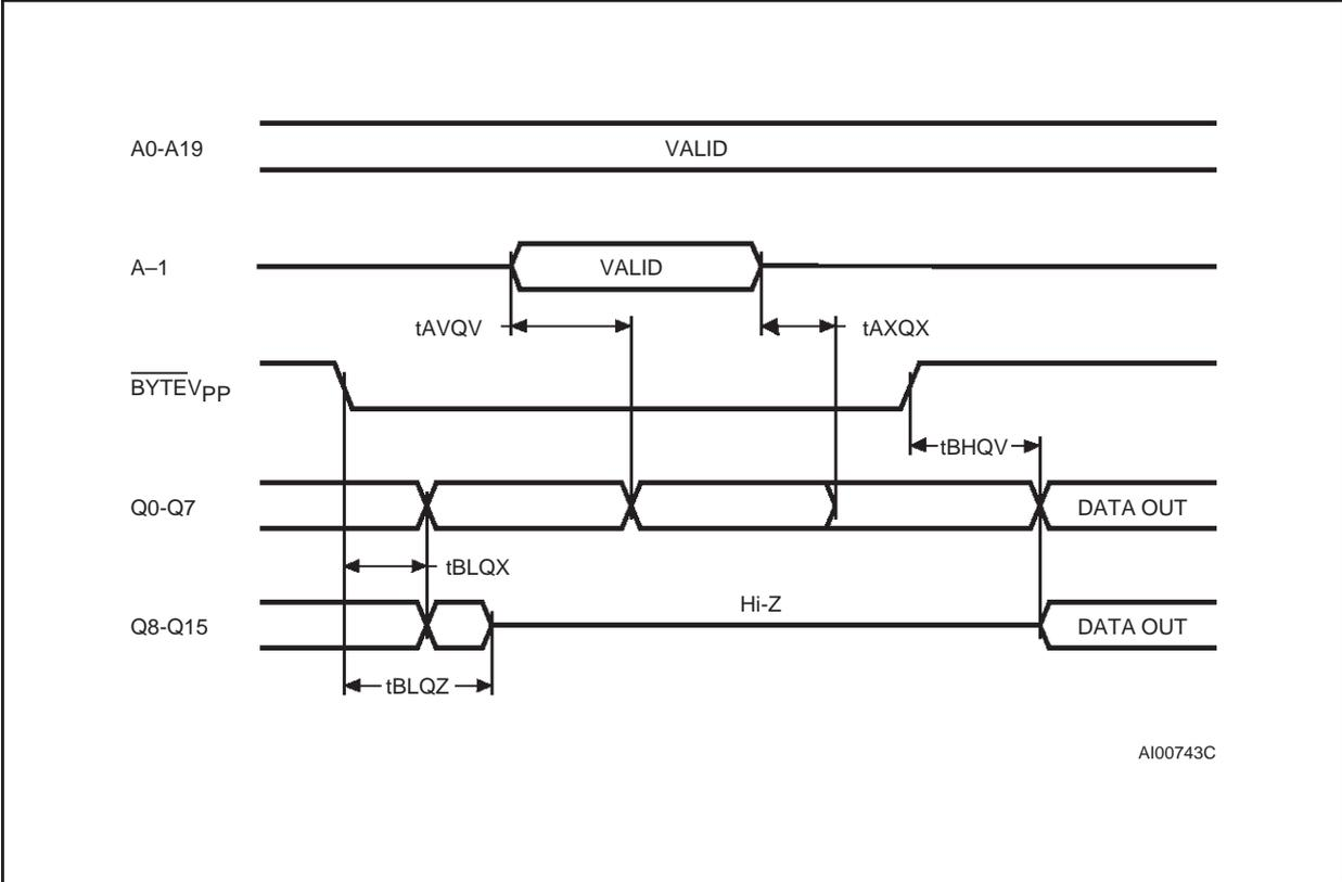
Note: Chip Enable ( $\bar{E}$ ) and Output Enable ( $\bar{G}$ ) =  $V_{IL}$ .
