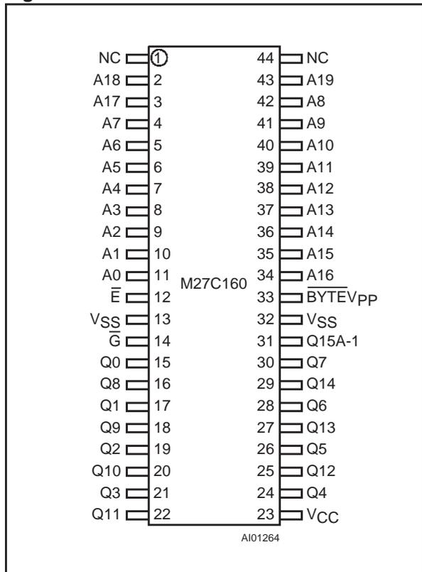
A new pattern can then be written rapidly to the device by following the programming procedure. For applications where the content is programmed only one time and erasure is not required, the M27C160 is offered in PDIP42, PLCC44 and SO44 packages.
