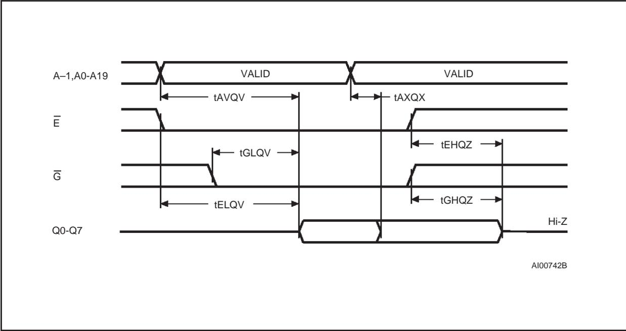
Note:  $\overline{BYTEV_{PP}} = V_{IL}$ .
