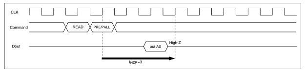
Write command to Precharge command interval (same bank): When the precharge command is executed for the same bank as the write command that preceded it, the minimum interval between the two commands is 1 clock. However, if the burst write operation is unfinished, the input data must be masked by means of DQM, DQMU/DQML for assurance of the clock defined by t<sub>DPL</sub>.
