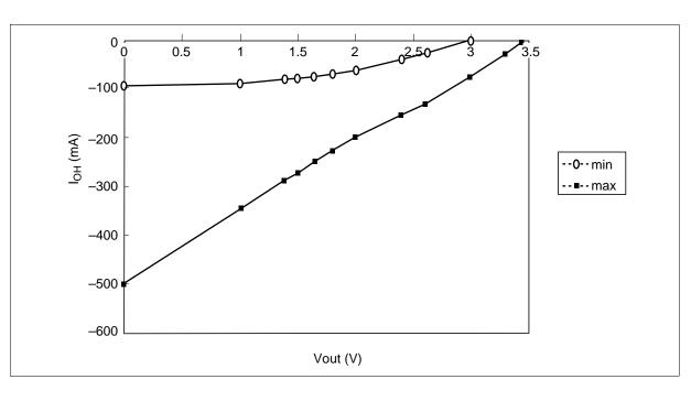
**DC Characteristics** (Ta = 0 to +70°C,  $V_{CC}$ ,  $V_{CC}Q = 3.3 \text{ V} \pm 0.3 \text{ V}$ ,  $V_{SS}$ ,  $V_{SS}Q = 0 \text{ V}$ ) (HM5264165F)
