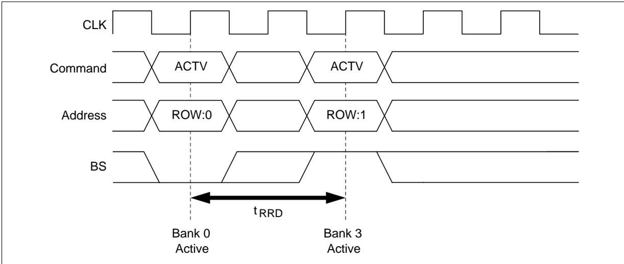
**Mode register set to Bank-active command interval:** The interval between setting the mode register and executing a bank-active command must be no less than  $I_{RSA}$ .
