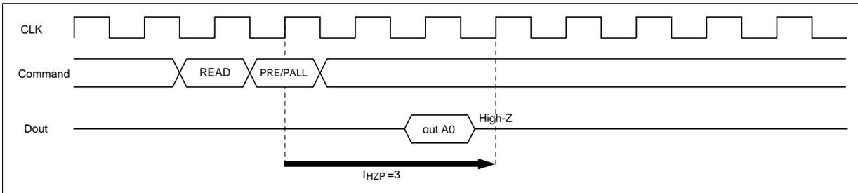
**Write command to Precharge command interval (same bank):** When the precharge command is executed for the same bank as the write command that preceded it, the minimum interval between the two commands is 1 clock. However, if the burst write operation is unfinished, the input data must be masked by means of DQM, DQMU/DQML for assurance of the clock defined by  $t_{DPL}$ .
