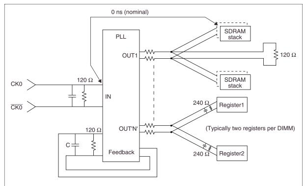
Notes: 1. The clock delay from the input of the PLL clock to the input of any SDRAM or register willI be set to 0 ns (nominal).
