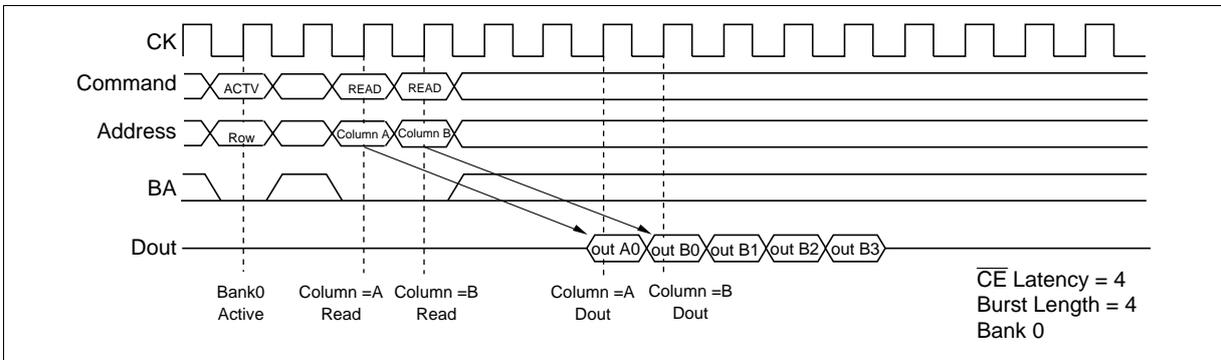
**2. Same bank, different ROW address:** When the ROW address changes on same bank, consecutive read commands cannot be executed; it is necessary to separate the two read commands with a precharge command and a bank-active command.
