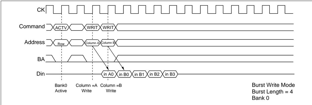
**2. Same bank, different ROW address:** When the ROW address changes, consecutive write commands cannot be executed; it is necessary to separate the two write commands with a precharge command and a bank-active command.
