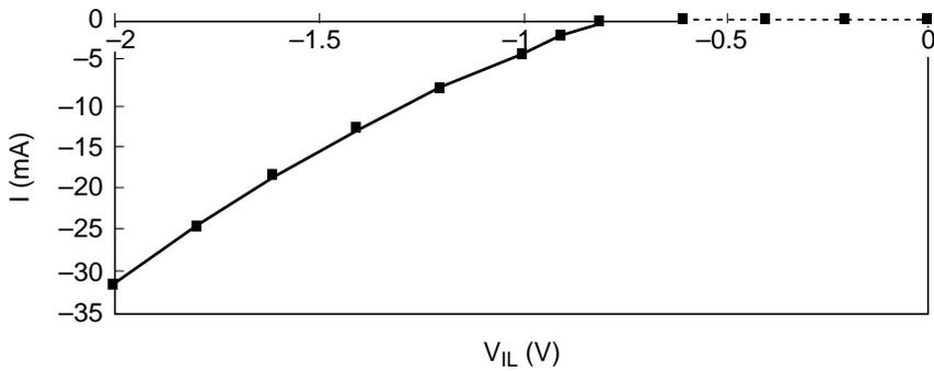
**Minimum  $V_{IH}$  Clamp Current** (referred to  $V_{CC}$ )
