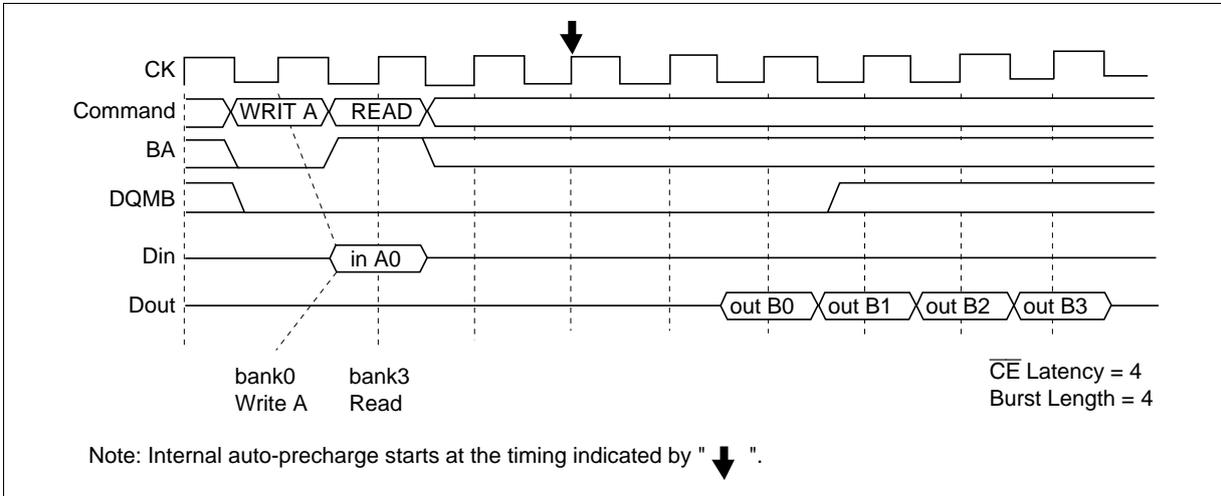
**2. Same bank:** The consecutive read command from write with auto precharge (the same bank) is illegal. It is necessary to separate the two commands with a bank active command.
