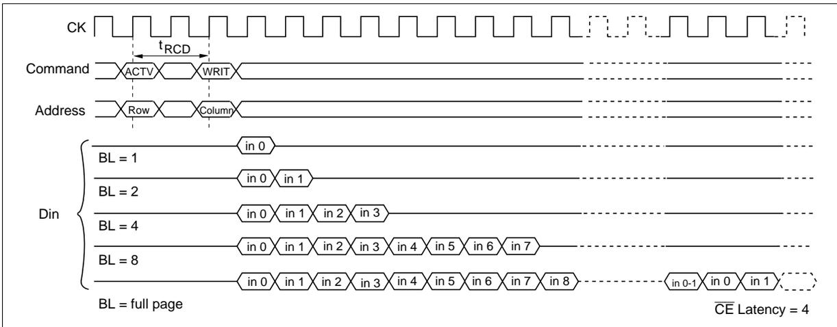
**2. Single write:** A single write operation is enabled by setting OPCODE (A9, A8) to (1, 0). In a single write operation, data is only written to the column address and the bank select address (BA) specified by the write command set cycle without regard to the burst length setting. (The latency of data input is 1 clock).
