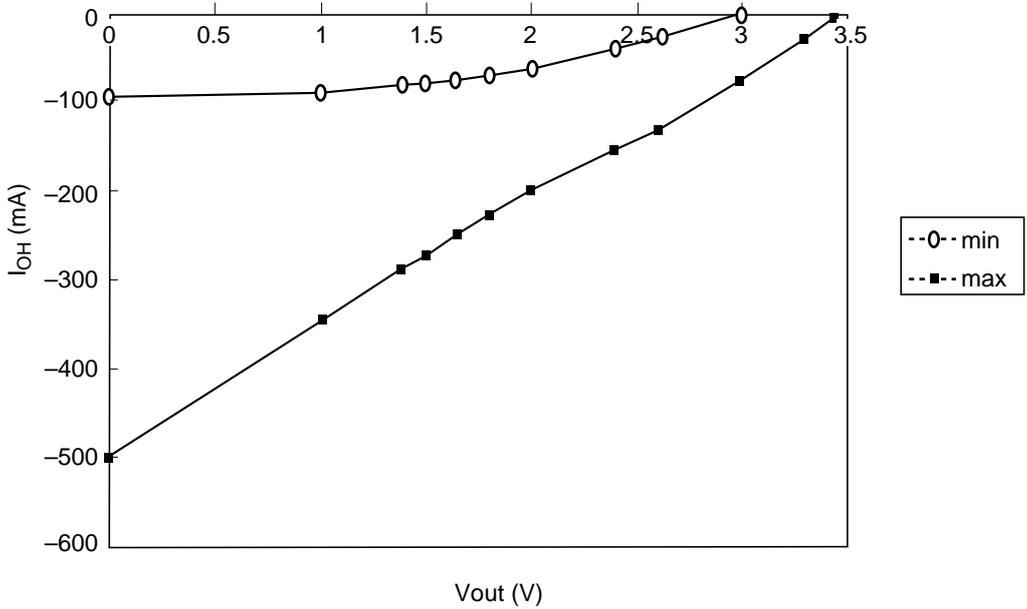
**DC Characteristics** ( $T_a = 0$  to  $55^\circ\text{C}$ ,  $V_{CC} = 3.3\text{ V} \pm 0.3\text{ V}$ ,  $V_{SS} = 0\text{ V}$ )
