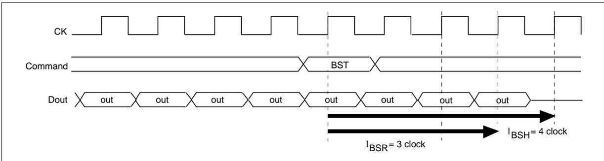
**Burst stop command at burst write:** The burst stop command (BST command) is used to stop data input during a full-page burst write. No data is written in the same clock as the BST command, and in subsequent clocks. In addition, the BST command is only valid during full-page burst mode, and is illegal with burst lengths of 1, 2, 4 and 8. And an interval of  $t_{DPL}$  is required between last data-in and the next precharge command.
