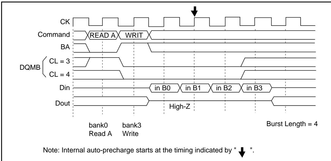
**2. Same bank:** The consecutive write command from read with auto precharge (the same bank) is illegal. It is necessary to separate the two commands with a bank active command.
