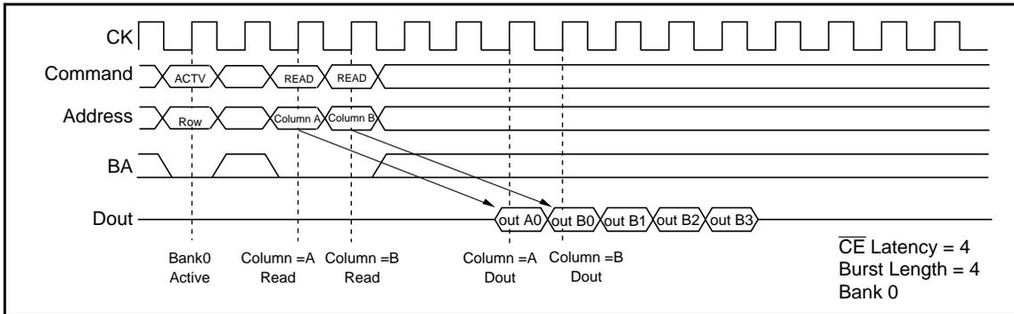
**2. Same bank, different ROW address:** When the ROW address changes on same bank, consecutive read commands cannot be executed; it is necessary to separate the two read commands with a precharge command and a bank-active command.
