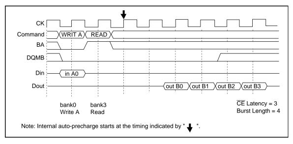
**2. Same bank:** The consecutive read command from write with auto precharge (the same bank) is illegal. It is necessary to separate the two commands with a bank active command.
