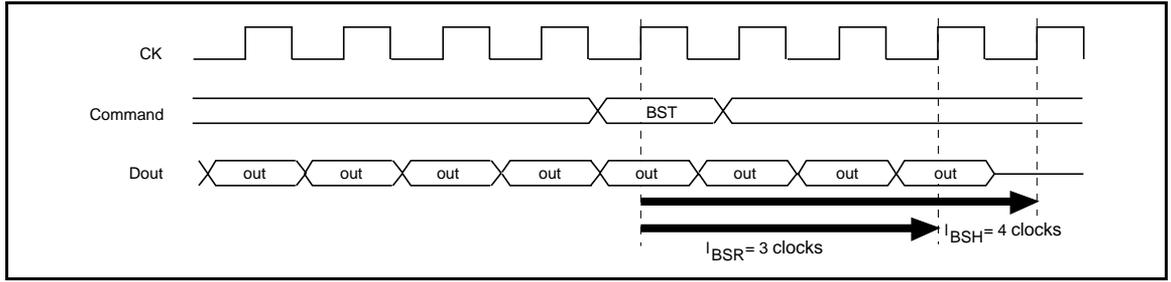
**Burst stop command at burst write:** The burst stop command (BST command) is used to stop data input during a full-page burst write. No data is written in the same clock as the BST command, and in subsequent clocks. In addition, the BST command is only valid during full-page burst mode, and is illegal with burst lengths of 1, 2, 4 and 8. And an interval of  $t_{DPL}$  is required between last data-in and the next precharge command.
