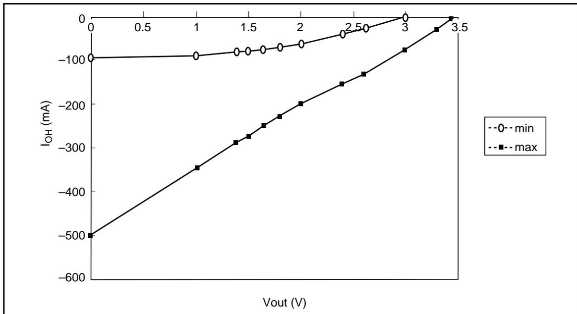
**DC Characteristics (Ta = 0 to 55°C, V<sub>CC</sub> = 3.3 V ± 0.3 V, V<sub>SS</sub> = 0 V)**
