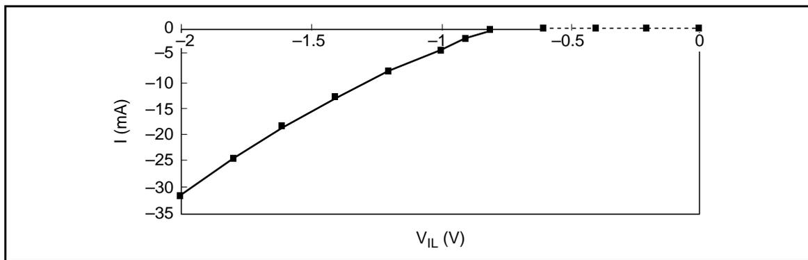
**Minimum  $V_{IH}$  Clamp Current (referred to  $V_{CC}$ )**
