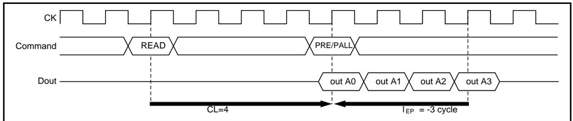
**READ to PRECHARGE Command Interval (same bank): To stop output data**
