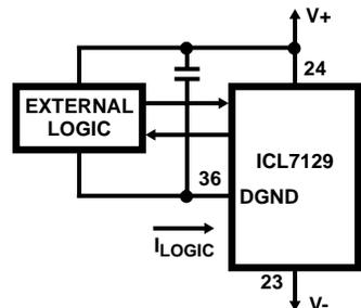
FIGURE 4. DGND SINK CURRENT
