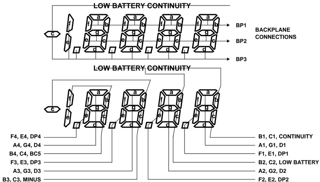
FIGURE 8. TRIPLEXED LIQUID CRYSTAL DISPLAY LAYOUT FOR ICL7129
