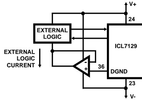
FIGURE 5. BUFFERED DGND
