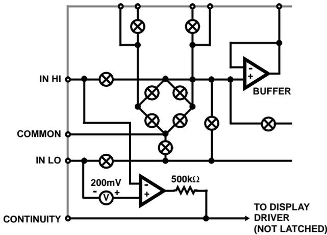
FIGURE 7. "INSTANT CONTINUITY" COMPARATOR AND OUTPUT STRUCTURE
