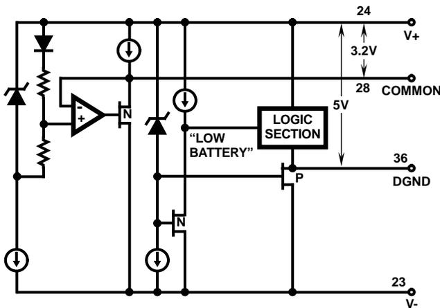
FIGURE 3. BIASING STRUCTURE FOR COMMON AND DGND
