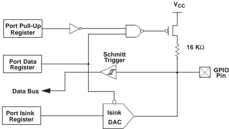
**Figure 5-9. Block Diagram of an I/O Line**
