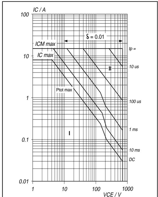
Fig.10. Forward bias safe operating area.  $T_{hs} = 25^{\circ}\text{C}$
