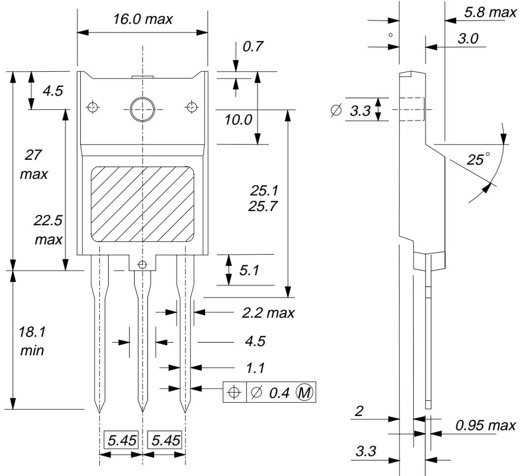
Fig.11. SOT399; The seating plane is electrically isolated from all terminals.
