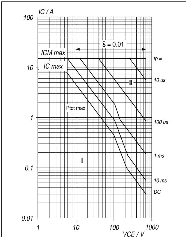
Fig.9. Forward bias safe operating area.  $T_{hs} = 25^{\circ}\text{C}$
