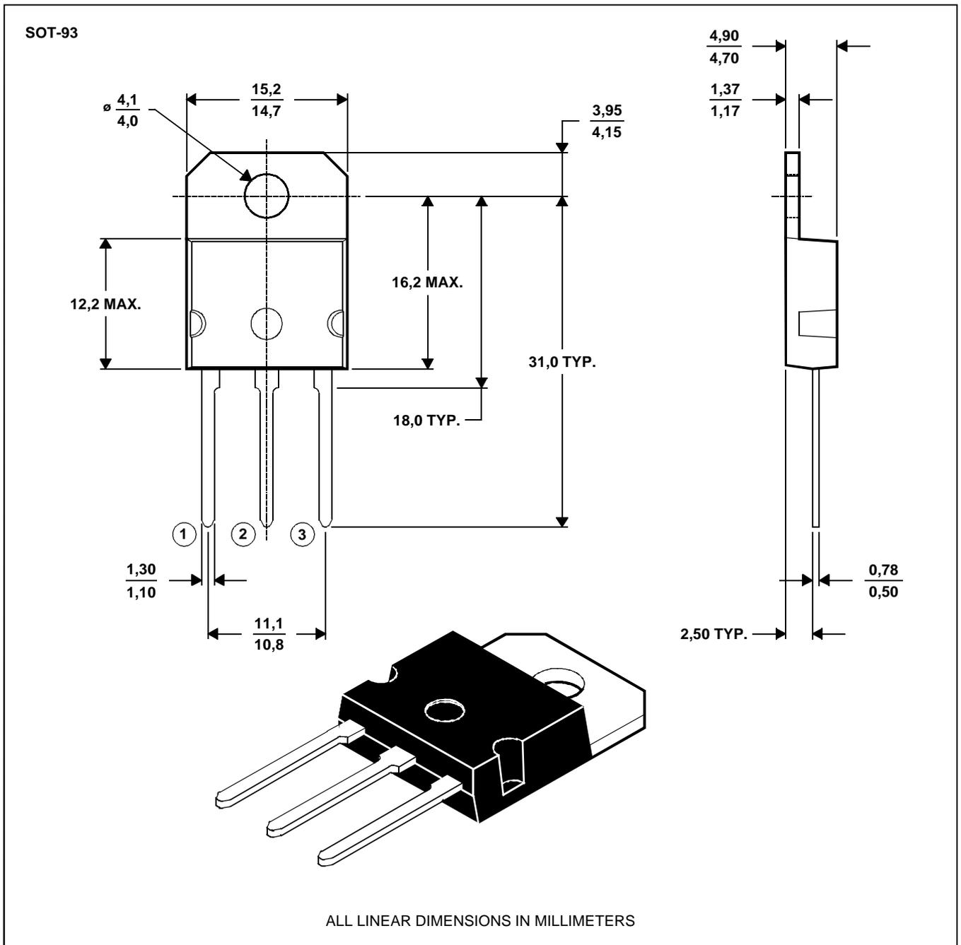
NOTE A: The centre pin is in electrical contact with the mounting tab.
