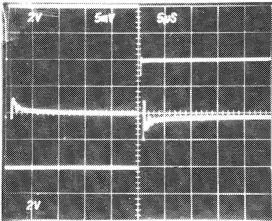
Top Trace: Output Signal; 2V/Div., 5μs/Div.
