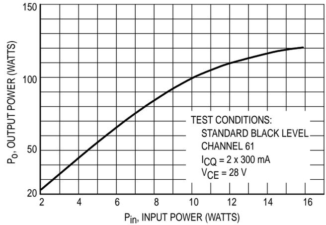
Figure 6. Peak Output Power versus Peak Input Power
