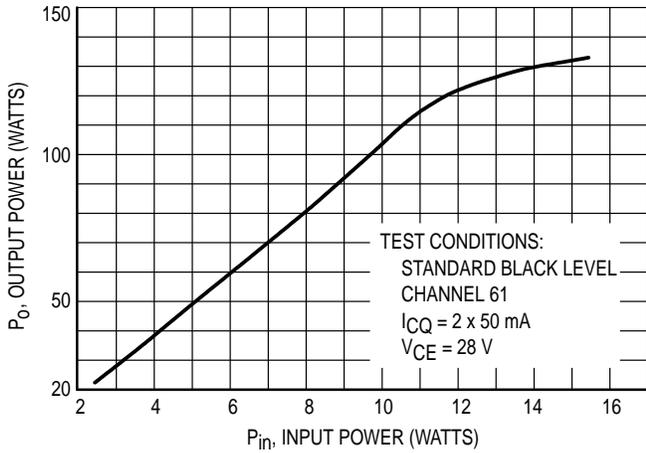
Figure 5. Peak Output Power versus Peak Input Power
