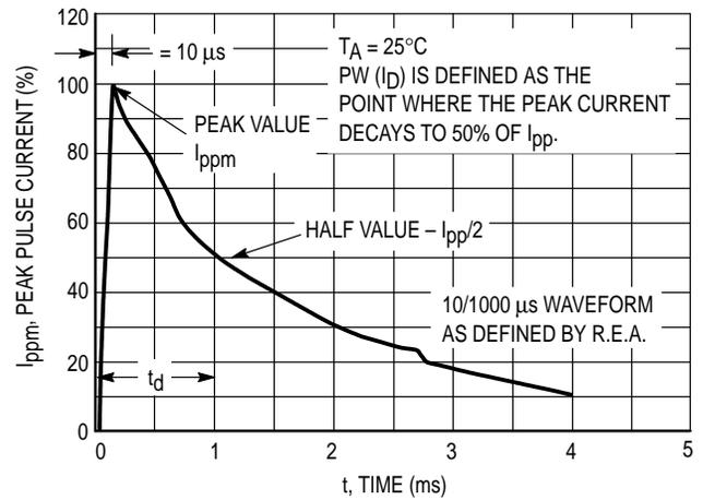
**Figure 4. Pulse Waveform 10/1000**
