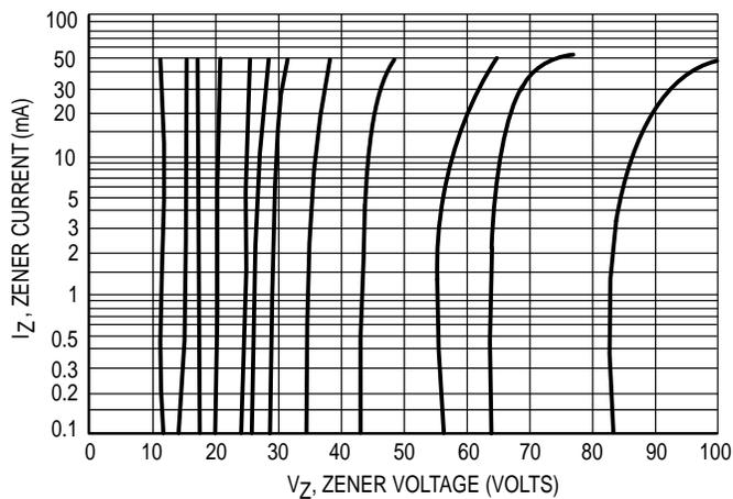
Figure 8.  $V_Z = 12$  thru 82 Volts
