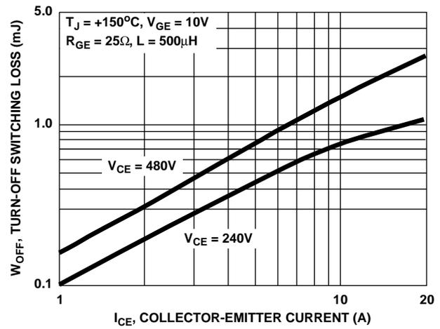
FIGURE 8. TURN-OFF SWITCHING LOSS vs COLLECTOR-EMITTER CURRENT
