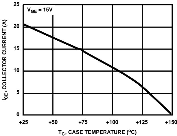
FIGURE 3. DC COLLECTOR CURRENT vs CASE TEMPERATURE
