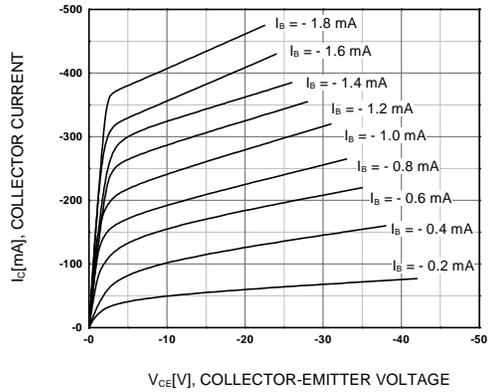
Figure 1. Static Characteristic
