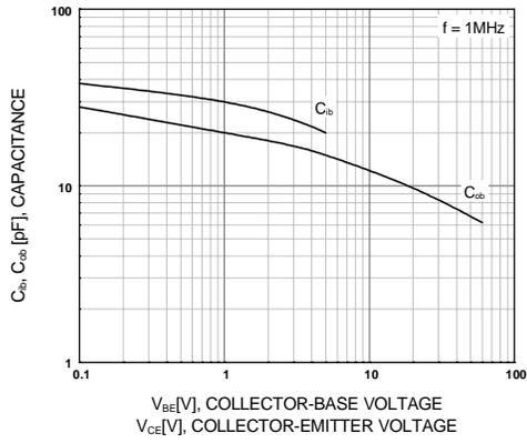
Figure 7. Input and Output Capacitance vs. Reverse Voltage
