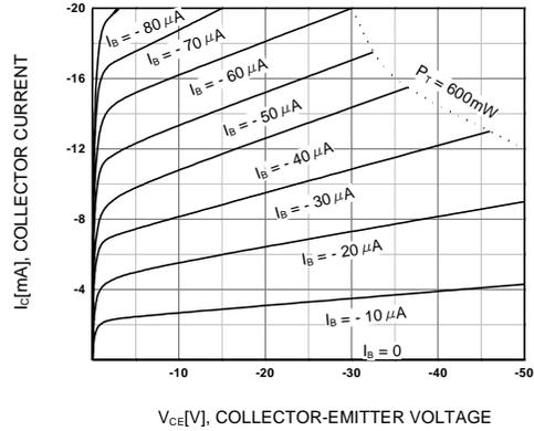
Figure 2. Static Characteristic
