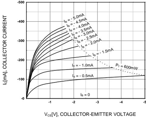
Figure 1. Static Characteristic
