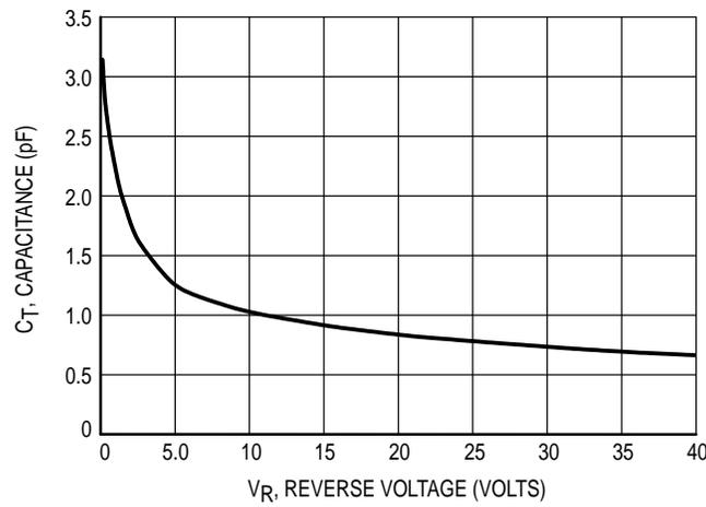
**Figure 3. Typical Capacitance**
