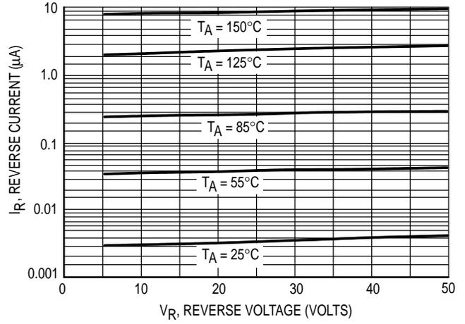
**Figure 5. Leakage Current**
