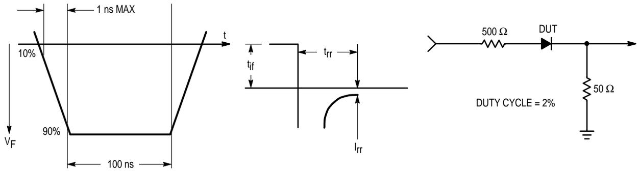
**Figure 1. Reverse Recovery Time Equivalent Test Circuit**
