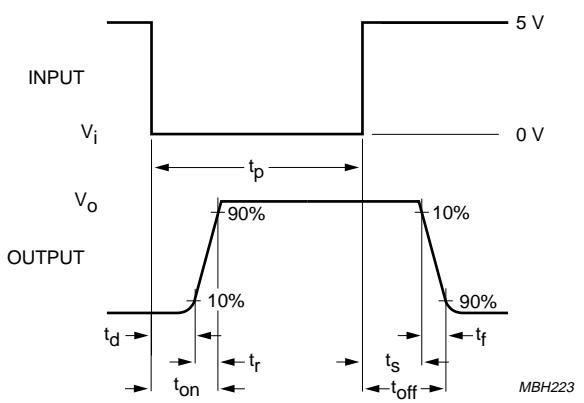
$t_r < 5 \text{ ns}$  (10% to 90%);  $t_p = 1 \mu\text{s}$ ;  $\delta = 0.02$ ;  $Z_i = 50 \Omega$ .
