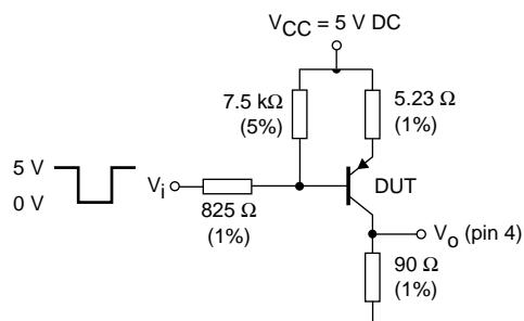
Fig.2 Switching times test circuit.
