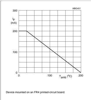
Fig.2 Maximum permissible continuous forward current as a function of ambient temperature.
