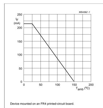
Fig.2 Maximum permissible continuous forward current as a function of ambient temperature.
