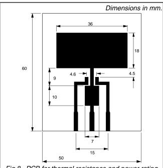
Fig.8. PCB for thermal resistance and power rating for SOT223.
