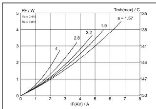
Fig.2. Maximum forward dissipation  $P_F = f(I_{F(AV)})$  per diode; sinusoidal current waveform where a = f form factor  $= I_{F(RMS)} / I_{F(AV)}$ .
