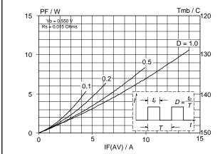
Fig.1. Maximum forward dissipation  $P_F = f(I_{F(AV)})$ ; square current waveform where  $I_{F(AV)} = I_{F(RMS)} \times \bigvee_{D} D$ .
