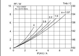
Fig.2. Maximum forward dissipation  $P_F = f(I_{F(AV)})$ ; sinusoidal current waveform where a = form factor =  $I_{F(RMS)} / I_{F(AV)}$ .
