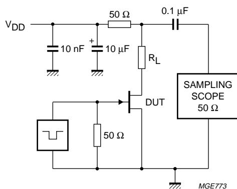
Fig.2 Switching circuit.
