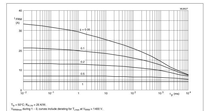
Fig.4 Maximum repetitive peak forward current as a function of pulse time (square pulse) and duty factor.
