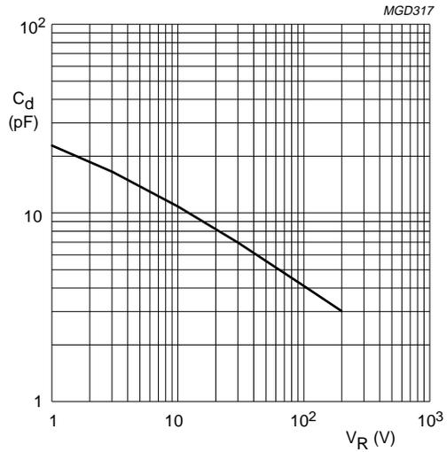
$f = 1 \text{ MHz}; T_j = 25 \text{ }^\circ\text{C}.$
