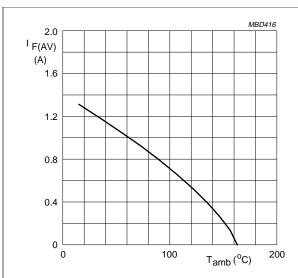
$a=1.42;\ V_R=V_{RRMmax};\ \delta=0.5.$  Device mounted as shown in Fig.8. Switched mode application.
