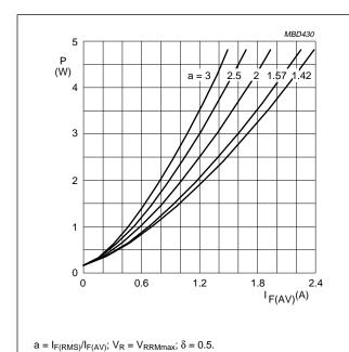
Fig.4 Maximum steady state power dissipation (forward plus leakage current losses,
