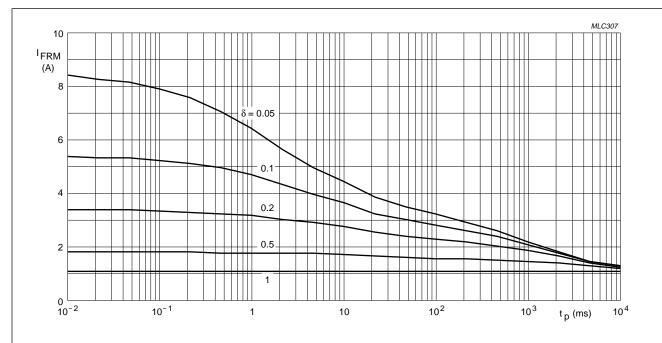
$T_{tp} = 55^{\circ}C$ ;  $R_{th j-tp} = 60$  K/W.
