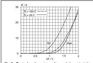
Fig.5. Typical and maximum forward characteristic;  $I_F = f(V_F)$ ; parameter  $T_j$
