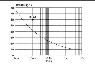
Fig.4. Maximum non-repetitive rms forward current.  $I_F = f(t_p)$ ; sinusoidal current waveform;  $T_j = 150^{\circ}\text{C}$  prior to surge with reapplied  $V_{RWM}$ .
