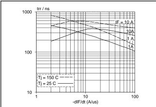
Fig.7. Maximum  $t_{rr}$  measured to 25% of  $I_{rrm}$ ;  $T_j = 25^{\circ}C$  and 150°C
