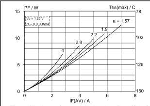
Fig.3. Maximum forward dissipation,  $P_F = f(I_{F(AV)})$ ; sinusoidal current waveform; parameter a = form factor  $= I_{F(RMS)}/I_{F(AV)}$ .
